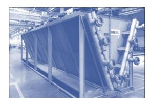
Ventilation can be handled by motor-fan groups or by motor and fan assembly, with direct or undirect transmission. Ventilation casing, frames and supporting legs can be of galvanized steel, liquid or powder painted carbon steel, stainless steel or galvanized steel.
